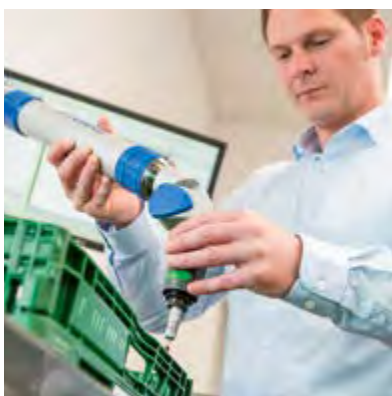
Check Using a Faro Measuring arm
